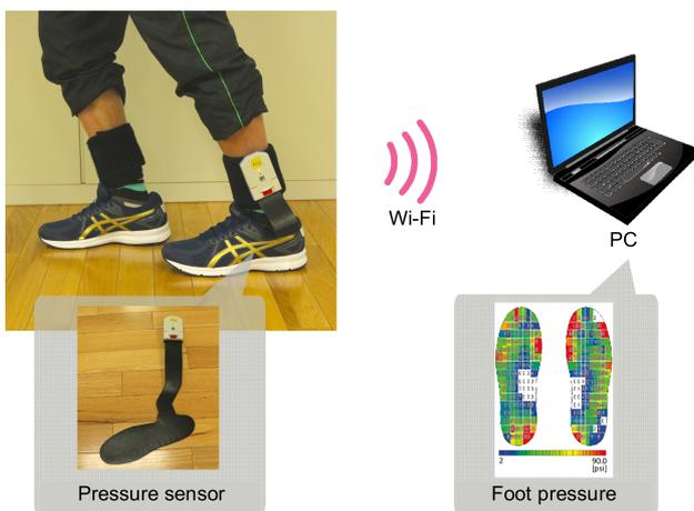
Fig. 1 System configuration.
