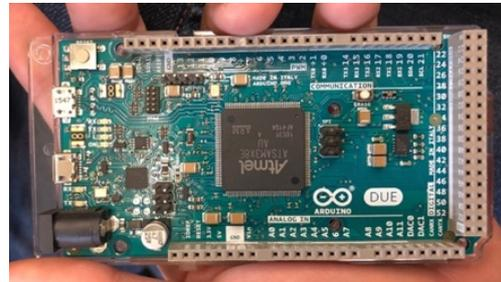
Fig.5 Arduino DUE.
