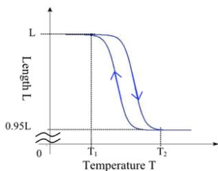
Fig. 3 Temperature Characteristics of SMA wire.
