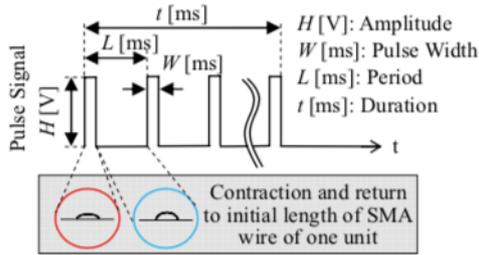
Fig. 2 Pulse signal for driving SMA wire.
