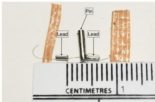
Fig. 4 Structure of SMA and pin.
