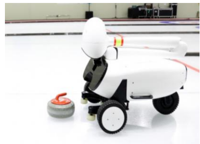
Figure 14. Demonstration game of the skip-thrower robot. Skip mode(top), throwing mode of grasping a stone(middle), releasing the stone(bottom)
