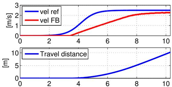
(a) Longitudinal velocity with only feedback controller
