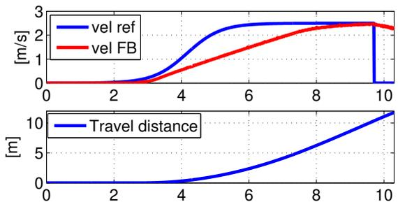
(b) Longitudinal velocity with feedback and feedforward controller
