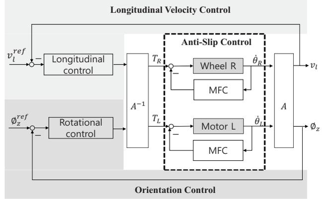
Fig. 3 Whole control algorithm of the mobile robot
