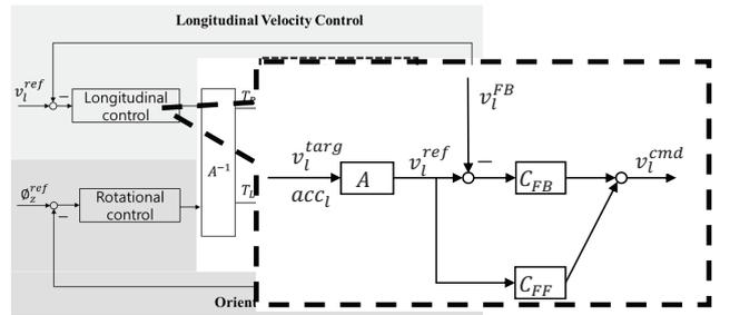
Fig. 4 Longitudinal velocity with feedback and feedforward controller
