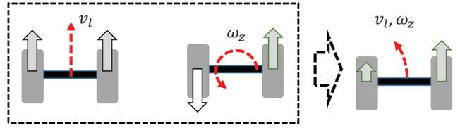
Fig. 2 Driving method on two-wheel driven mobile robot
