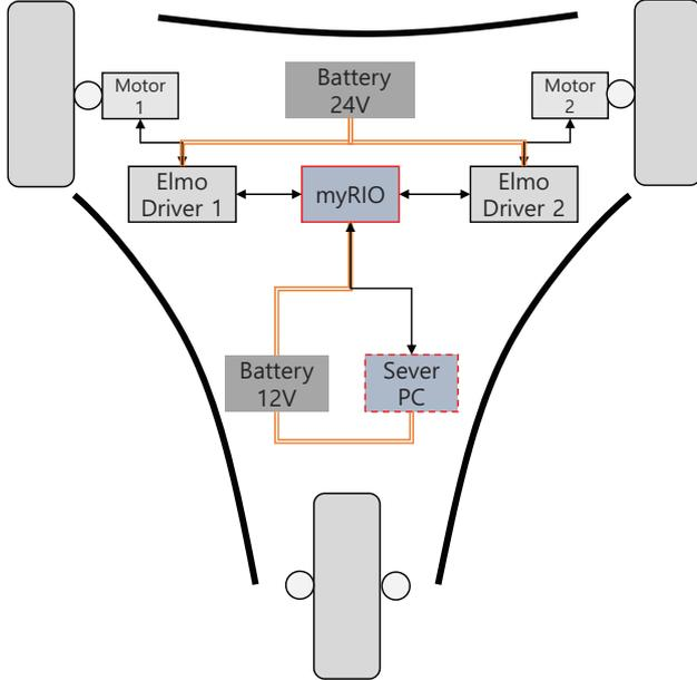
(b) Electronic structure of the mobile robot
