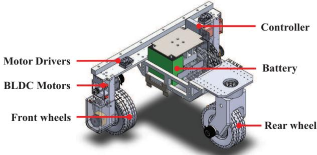
(a) Mobile robot prototype
