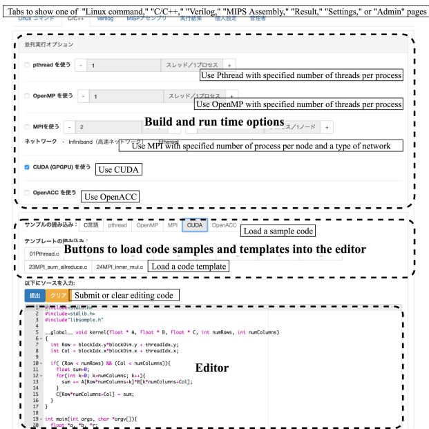
Fig. 5 Coding environment of FEHA. Learners input a code from the screen and submit it with the build and runtime options.
