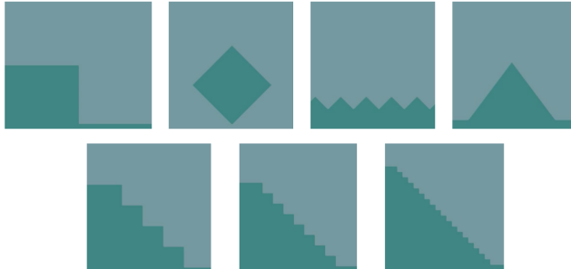
Fig. 3 Different floor shapes used in our simulations. In the first row, from left to right, we name them L , square , zigzag and triangle . In the second row, from left to right, we name them stair1 , stair2 and stair3 .
