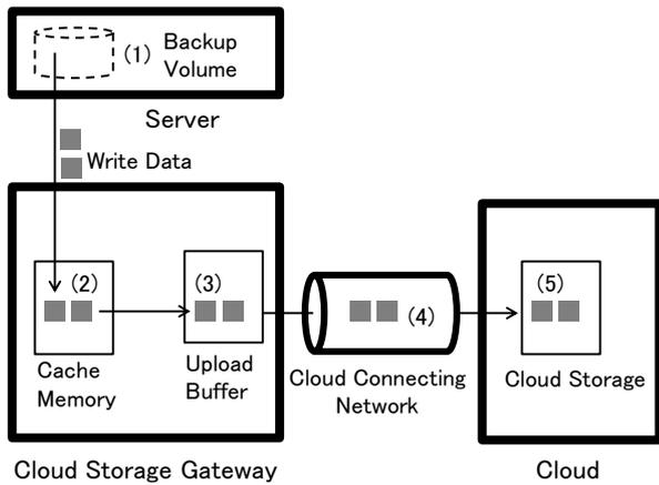
Figure 7 Cloud-based Data Backup System Model
