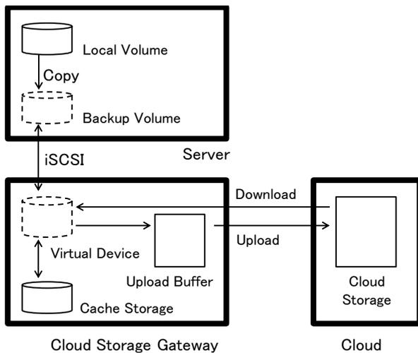
Figure 2 Cloud-based Data Backup System
