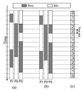
Fig. 2 Illustration of the inter-TLP estimation mechanism. (a) Utilization of three processors P1, P2, and P3. (b) Utilization quantized in time slots. (c) Concurrency for each time slot.
