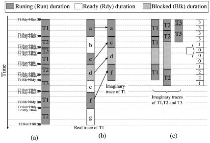
Fig. 3 Illustration of the intra-TLP estimation mechanism. (a) Three tasks, T1, T2, and T3 being executed on the same processor. (b) Real trace and imaginary trace of T1. (c) Imaginary traces of all tasks and the concurrency for each time slot.
