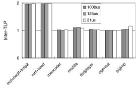
Fig. 5 Estimated inter-TLP for three different sizes of time slot.
