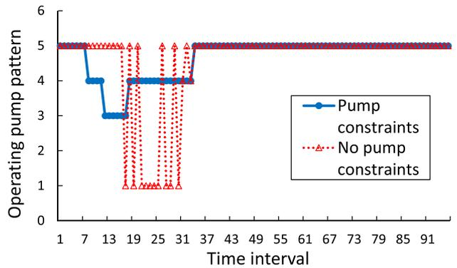
Fig. 8 Example of optimal pump operations at a pump station over 96 time intervals.
