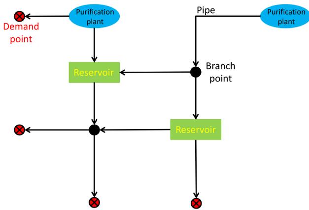
Fig. 1 Sketch of overall water distribution network of the water supply utility.
