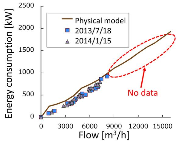
Fig. 2 Comparison between the energy consumption curve based on the physical model and past actual values at a typical pump station.
