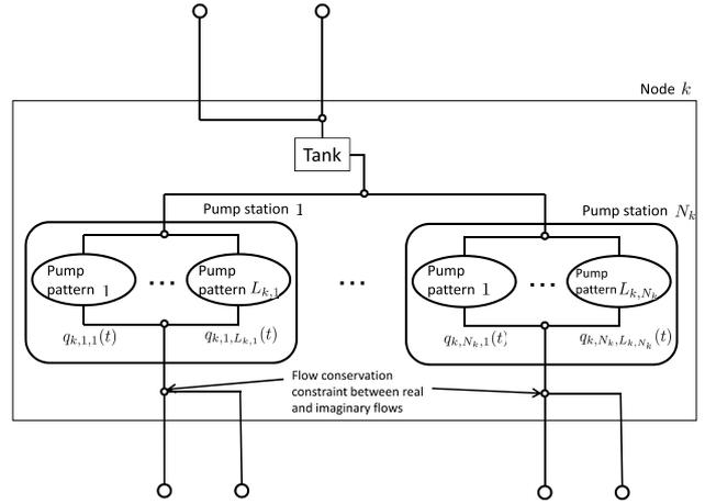
Fig. 4 Overview of the imaginary flow at the node  $k \in \mathcal{P} \cup \mathcal{R}$  in the time interval  $t$ .
