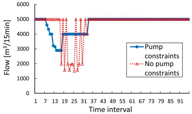
Fig. 7 Example of optimal water distribution from a pump station over 96 time intervals.
