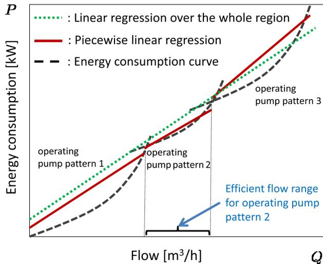
**Fig. 3** Conceptual diagram of the energy consumption curve developed by pump modeling (dashed line) and two approximations by the linear regression over the whole flow range (dotted line) and the piecewise linear regression over each of the efficient flow ranges (solid line).
