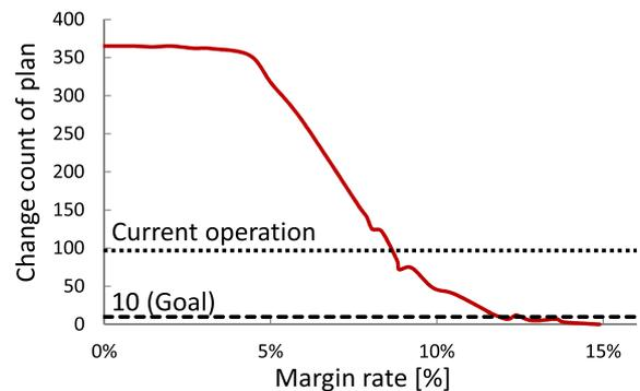
Fig. 6 Relation between the margin rate of gross water supply quantity for the total amount of water demand and the change count of the original plan with RO.
