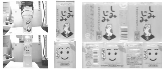
(a) Original image (b) Piece image (c) Developed image top: can bottom: square type PET bottle 図 4 投影画像の生成
