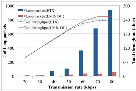
Fig. 3 Loops/throughput with various CBR rate.
