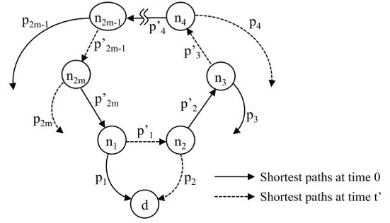
Fig. 1 The general case of routing loops.
