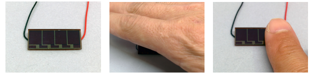
Fig. 2 A PV module (left figure) and examples of blocking actions using PV modules. When several fingers or the palm approaches and covers the whole PV module, the illumination level falls enough to be detected as interruption of energy supply (middle figure). Many objects are opaque and can replace the fingers or palm. Considering partial shadowing, finger-touch on one PV cell also decreases energy generation and is detected as energy blocking (right figure).
