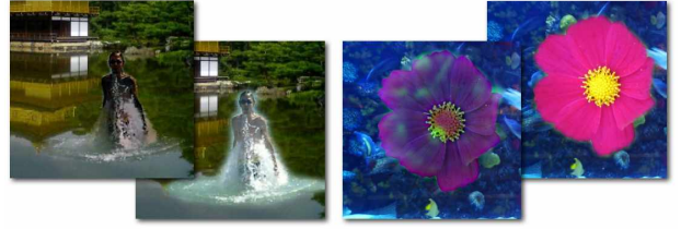
Figure 2: Poisson blending. Two examples with Poisson optimization importing the source image gradient (left image of each example), and with just alpha matting (right image on each example).
