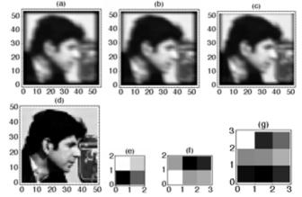
**Fig. 1**. (a): Test image obtained from a true image of (d) by convolving the three blurs of (e), (f), and (g). The image size is  $44 \times 45$ . (b): Image restored by removing the blur of (e). (c): Image restored by removing blurs of (e) and (f). (d): Image restored by removing blurs of (e), (f), and (g).
