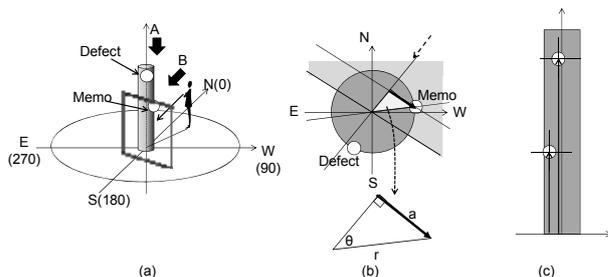
Fig.4 Calculation of defect location in reference step
