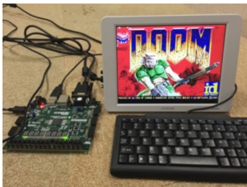
Figure 3: The snapshot of DOOM running on Nexys4 DDR FPGA board. DOOM is the first FPS game and very famous one.
