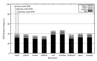
Fig. 8 Overall dynamic energy of proposed BTB (4-way and 2,048-entry BTB).
