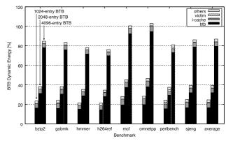
Fig. 6 Overall dynamic energy of proposed BTB (4-way and 128-entry victim BTB).
