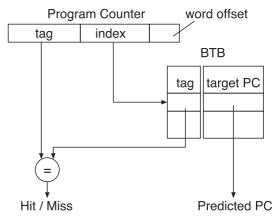
Fig. 1 Branch target buffer.
