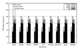
Fig. 11 Influence of I-cache capacity on overall static energy of proposed BTB.
