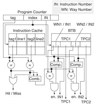
Fig. 2 Proposed mechanism.
