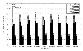
Fig. 12 Overall dynamic energy of related mechanisms.
