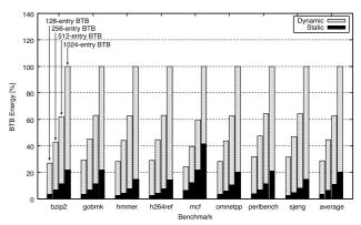
Fig. 5 Overall dynamic and static energy of conventional BTB.
