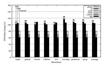
Fig. 13 Overall static energy of related mechanisms.
