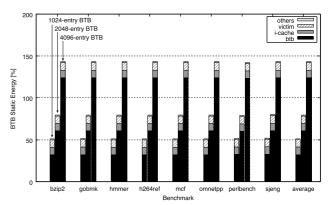
Fig. 7 Overall static energy of proposed BTB (4-way and 128-entry victim BTB).
