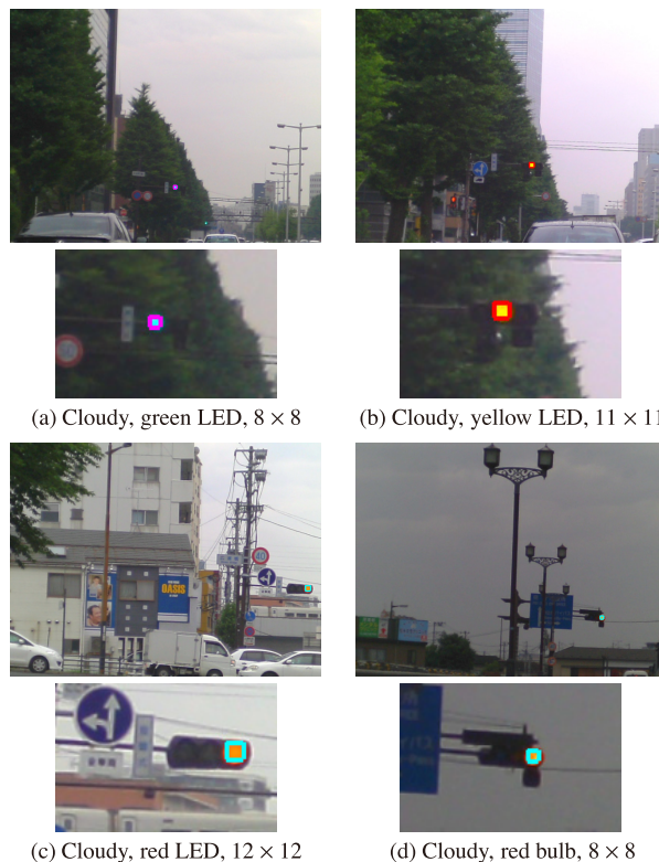
Fig. 9 Results of traffic light detection in various conditions using the proposed method.
