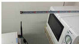
Fig. 5 USRP deployed 0.3 m away from the front door of microwave oven.
