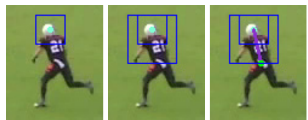
(a) Head region tracked by the head tracker. (b) Upper body region (larger rectangle) used for poselet-regressor. (c) 2D spine estimated by poselet-regressor to estimate pelvis position.
