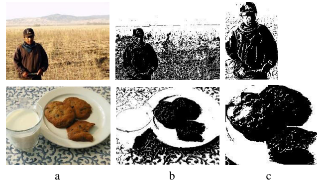
Figure 7. Results Produced by Belief Propagation Algorithm. (a) Input image. (b) Results produced by BP without masks. (c) Results produced by BP only on the foreground objects.
