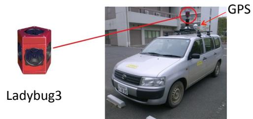
Fig. 3 Measurement vehicle equipping an omnidirectional camera (Ladybug 3) and GPS.
