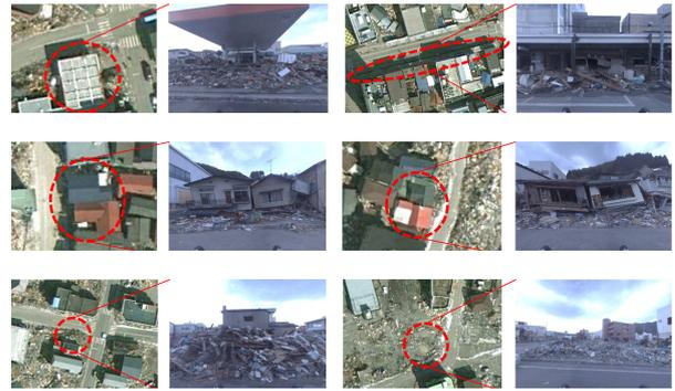
**Fig. 20** Example aerial and street-view images. There are many cases in which aerial images and street-view images give complementary information about the land surface condition. For example, the areas covered by the building roof (the top and second row), stacked objects (the bottom row) are best viewed from the street.
