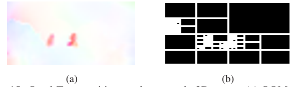
Fig. 15: Quad-Tree partition on the example 3D scene: (a) OOM; (b) Quad-Tree partition. (Copyrighted by Springer LNCS [57])
