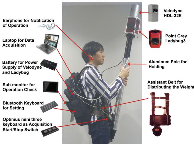
Fig. 3: Photo of Velobug system actually equipped on a cartographer
