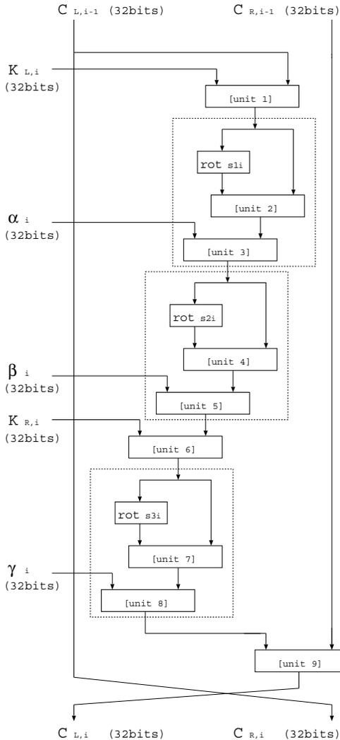
Fig. 1 The round function of M8.
