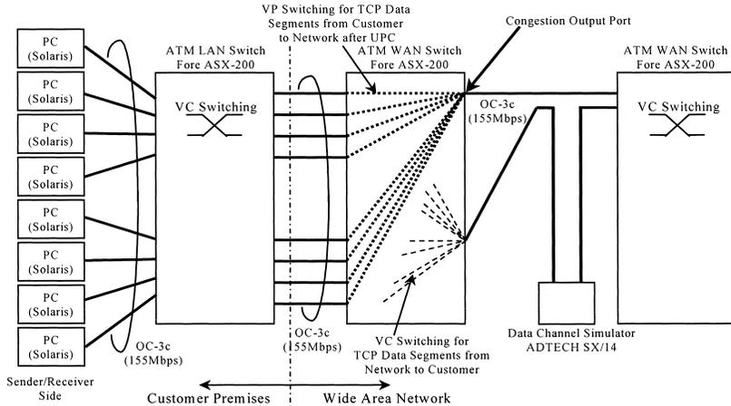
Fig. 2 Experimental configuration.
