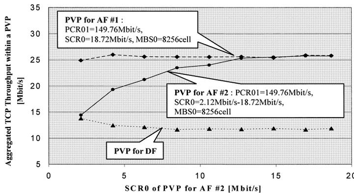
Fig. 6 Effect of SCR0 with RTT = 80 ms.
