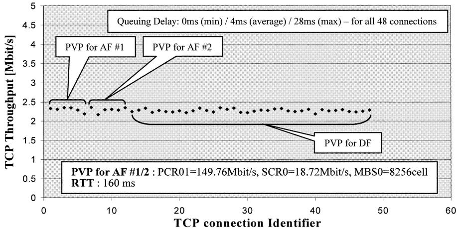
Fig. 5 Each TCP throughput under PVPs for AF and DF PHBs with RTT = 160 ms.
