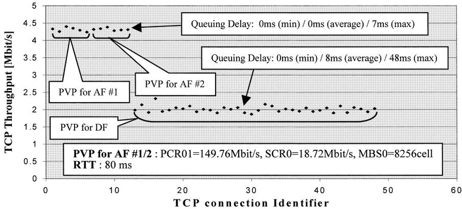
Fig. 3 Each TCP throughput under PVPs for AF and DF PHBs with RTT = 80 ms.
