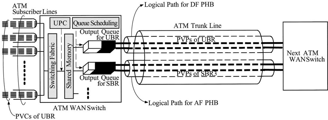
Fig. 1 Mapping strategy of AF/DF PHBs to ATM PVP connections.
