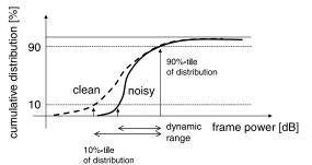
Fig. 1 Cumulative distribution of frame power and the dynamic range of a signal. When the noise signal masks the speech signal, the lower bound of the distribution of frame powers becomes higher.
