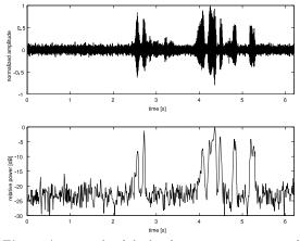
Fig. 3 An example of the log frame power sequence of a sub-band (3.0–3.5 kHz) when human speech like noise of 1,024 superpositions is added with the global SNR of 5 dB. Full-band waveform (upper) and sub-band log frame power sequence (lower).
