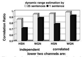
Fig. 9 Correlation coefficients between predicted and actual recognition accuracy calculated under various conditions (WGN: white Gaussian noise, HSN: Human-speech-like noise).
