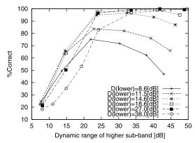
Fig. 6 Recognition performance as a function of the sub-band dynamic range of 0.5–1.0 kHz, i.e., the higher sub-band, when noise also exists in 0– 0.5 kHz, i.e., the lower sub-band, with SNR of D (lower).
