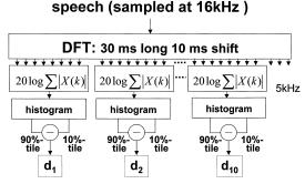
Fig. 2 Calculation method for sub-band dynamic range.
