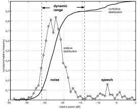
Fig. 4 Histogram and cumulative distribution of the sub-band log frame powers of the noisy speech given in Fig. 3.
