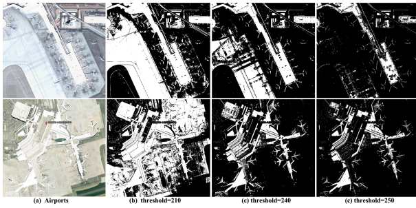
Fig. 6 For white aircrafts, constant multi-thresholds are suitable for segmenting aircrafts from different airport images.
