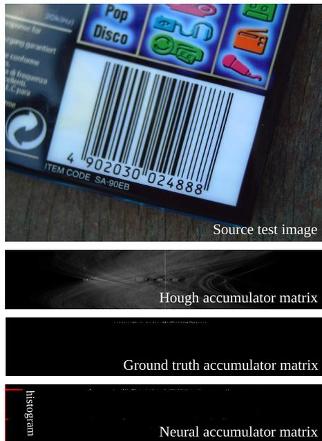
**Fig. 4** An example showing the accumulator matrices generated by the angle detection phase for an image in the *ArTe-Lab 1D Dataset*. In the right part of the figure, from top to bottom: the original accumulator matrix  $A_H$ ; the ground-truth accumulator matrix in which elements denoting barcode bars in the original image have been assigned an high intensity value; the neural accumulator matrix  $A_N$  generated by our trained neural model for  $A_H$ .
