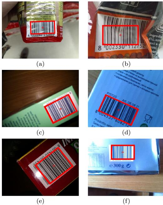
**Fig. 1** Examples showing the bounding boxes automatically identified by the proposed method for arbitrary rotated 1D barcodes in images acquired using smartphones. The results produced by the proposed method are satisfying even when the 1D barcodes are warped, occluded or partially illegible due to reflections.
