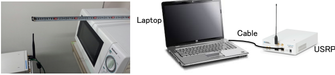
Fig. 6 USRP and laptop connected via an ethernet cable in each measurement set.
