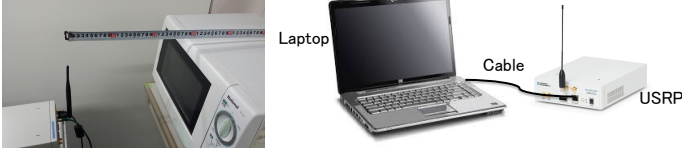
Fig. 5 USRP deployed 0.3 m away from the front door of microwave oven. Fig. 6 USRP and laptop connected via an ethernet cable in each measurement set.
