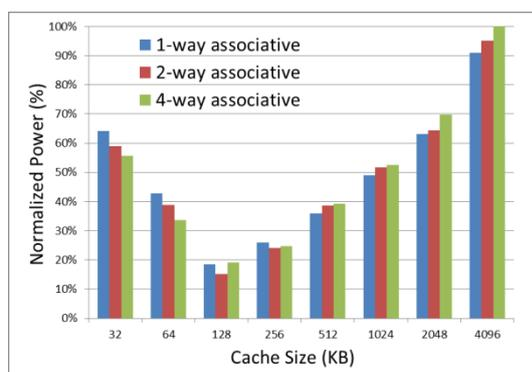
Figure 3: Power consumption (Bzip2 application)
