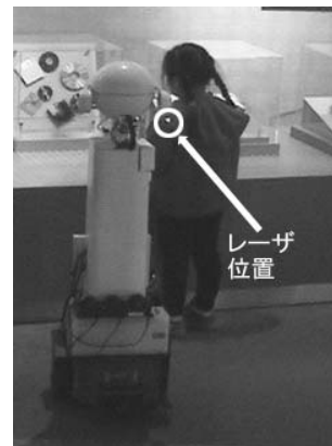
図 14 来館者の肩にレーザが遮られている場面 Fig. 14 The scene where the laser spot was obstructed by visitor's shoulder.
