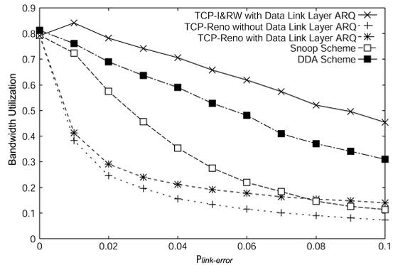
Fig. 9 Bandwidth utilization on the satellite link.
