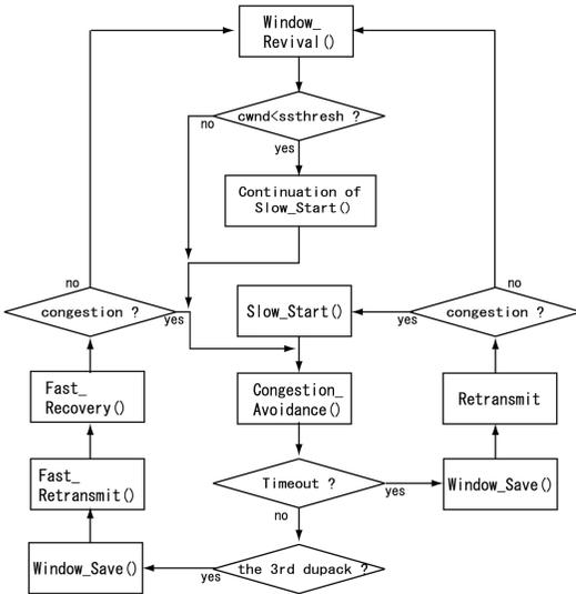
Fig. 1 Flowchart of TCP-I&RW sender operation.
