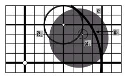
Fig. 4 Snapping candidates and fuzzy cursor in multi-resolution grid system.
