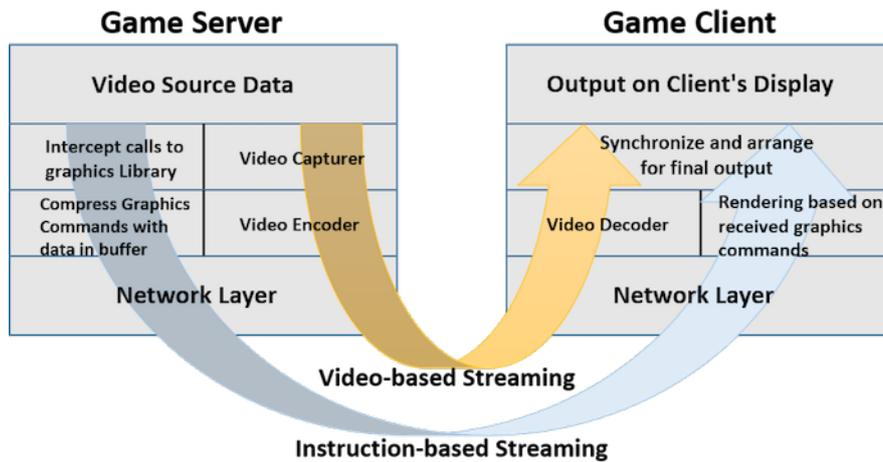
Fig. 1 An overview of our proposed hybrid-streaming model
