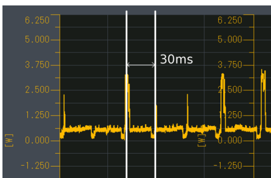
Figure 8: Power waveform with OSCAR power control
