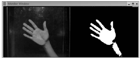
図13 カメラからの取得画像(左)と背景差分画像(右) Fig. 13 A captured image (left) and its digitized image (right).
