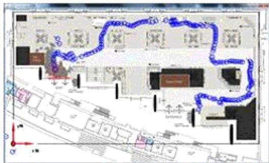
Fig. 21 Trajectory Path Estimated Using a 16m Grid Size RSSI Map
