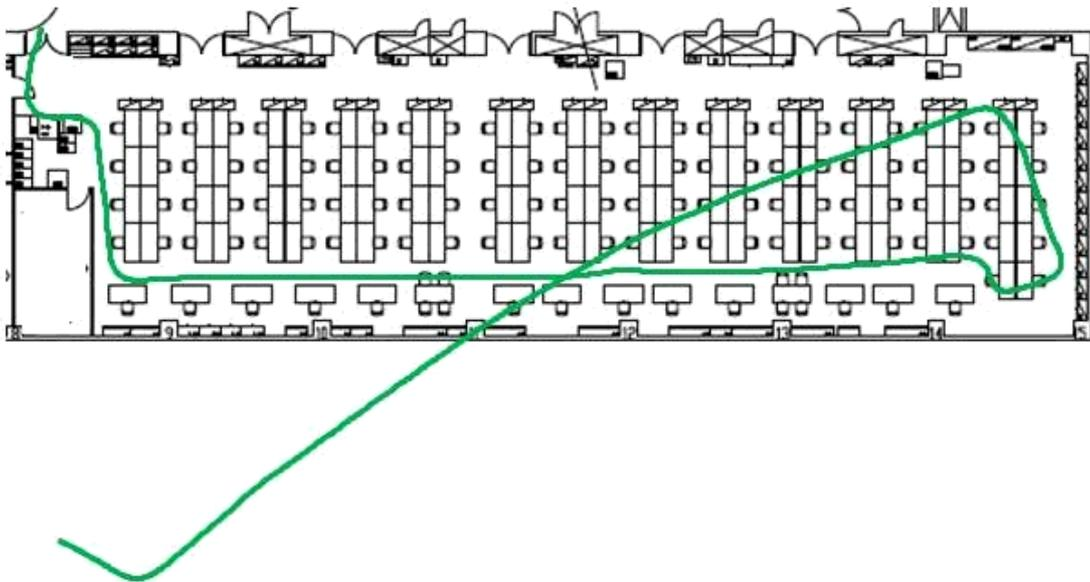
Fig. 12 A Sample of Trajectory Path Estimated Using the PDR
