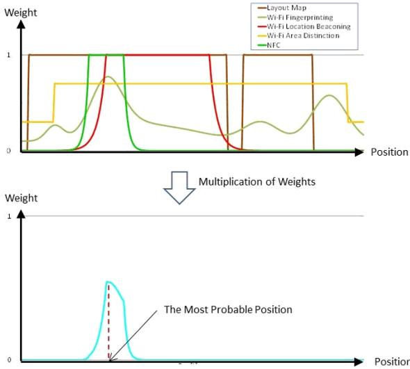
**Fig. 7** Theory of Weighting for the Particle Filter
