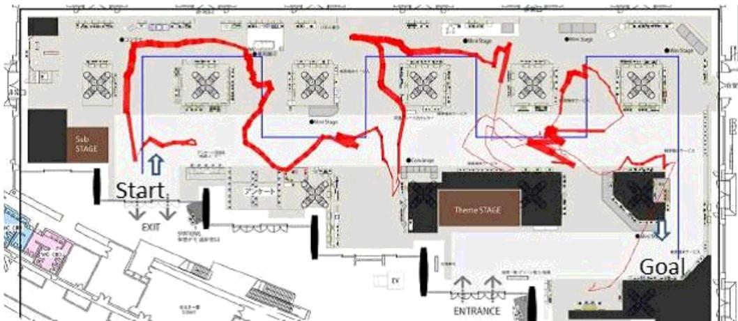
Fig. 15 A Sample of Trajectory Path Estimated by Combining PDR, Wi-Fi Fingerprint and Layout Map
