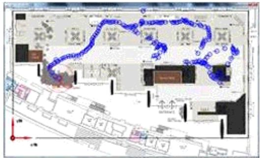
Fig. 20 Trajectory Path Estimated Using a 6m Grid Size RSSI Map
