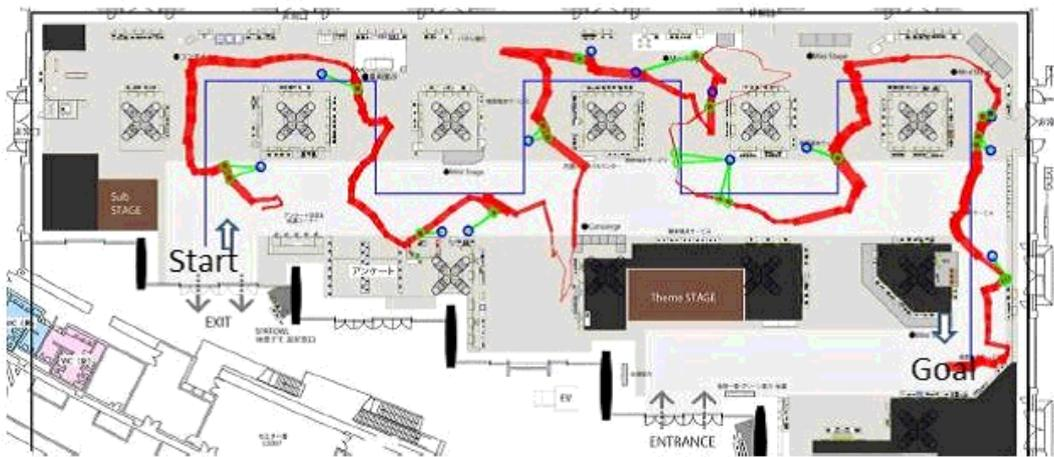
Fig. 16 A Sample of Trajectory Path Estimated by Combining PDR, Wi-Fi Fingerprint, Layout Map, Wi-Fi Location Beacon and NFC
