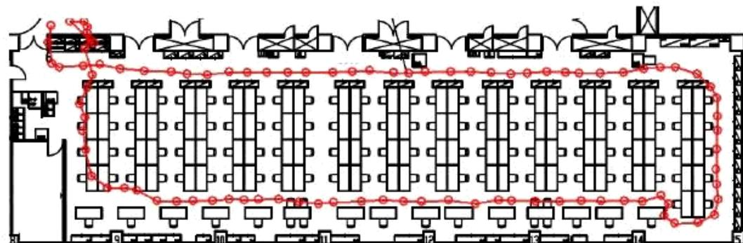
Fig. 13 A Sample of Trajectory Path Estimated by Combining PDR, Wi-Fi Fingerprinting and Layout Map
