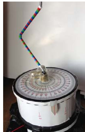
Figure 18: Standard Positioned 3D marker Rotation (0, 0, 45) on the Turn Table.
