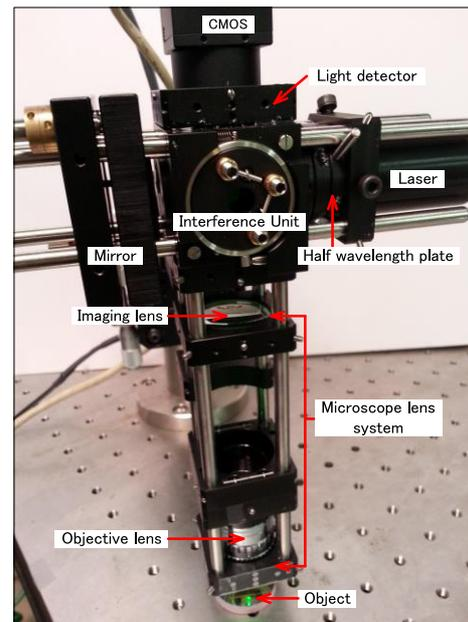
Fig. 2 Appearance of proposed 3D microscope.
