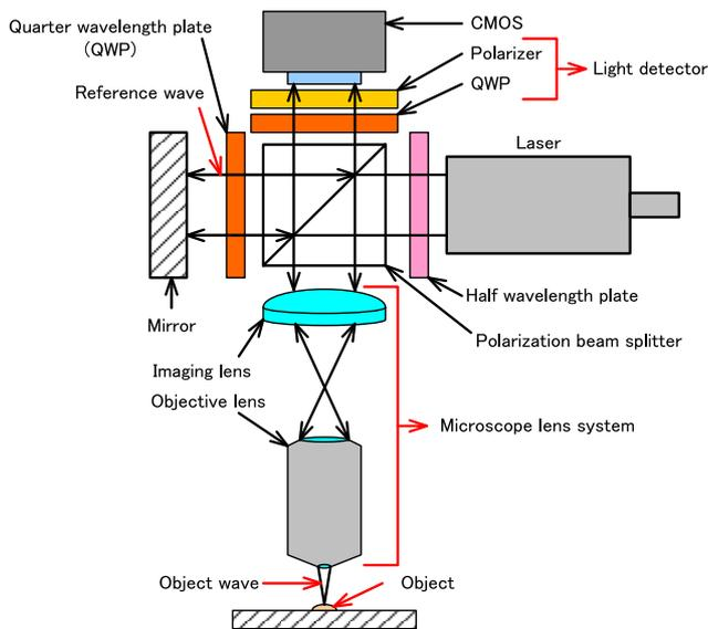
Fig. 1 Structure of proposed 3D microscope.
