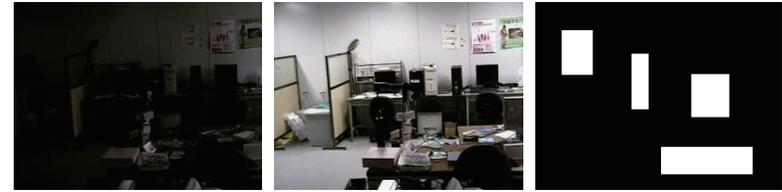
**Fig. 5** Experimental data for background estimation. The left indicates an observed image, the center is the model background image, and the right is hypothetic foreground-candidate regions which are manually established for this experiment.
