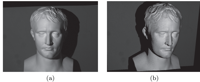
Fig. 4 (a) One of the three images captured for photometric stereo. (b) Measured shape by triangulation.
