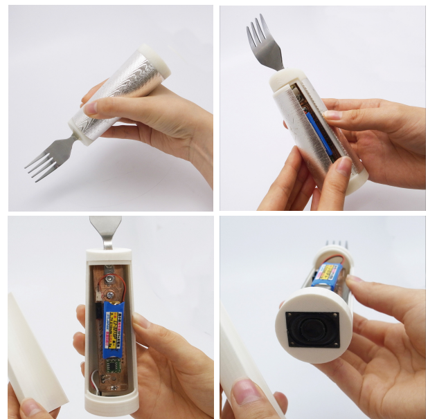
Fig. 5 Fork-type device. Grip size: 120 mm circumference and 105 mm height).
