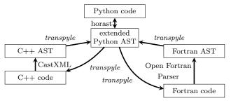
Figure 3 Diagram showing responsibilities of various modules used in our transpilation framework
